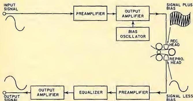
Fig. 1. Block diagram of the direct-record system described.
