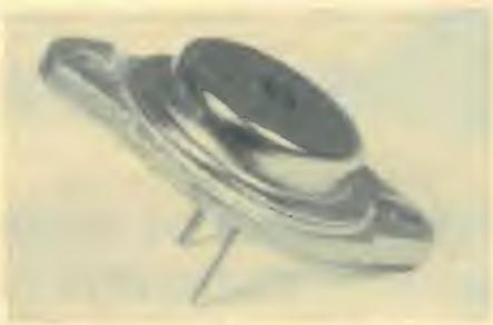
specifications include a minimum gain of 10 at 25 amps,  $V_{CE0}$  of 40-80 volts,  $V_{CEX}$  of 40-80 volts, and  $V_{CE0}$  of 30-50 volts.
