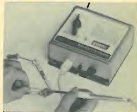
dering pen and heat capsule with coaxial connector, "Select-A-Temp" control unit, and three of the most widely used Princess threaded soldering nibs.
