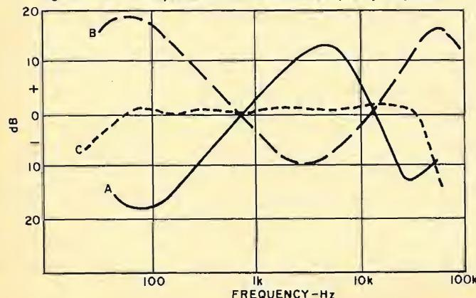
The reproduce signal at the playback head is shown minus the bias oscillator signal. Most of this is lost due to the spacing of the reproduce head gap. It is not sufficiently small so as to reproduce the high-frequency bias signal. The remainder of the bias signal is usually removed by a simple RC filter.
