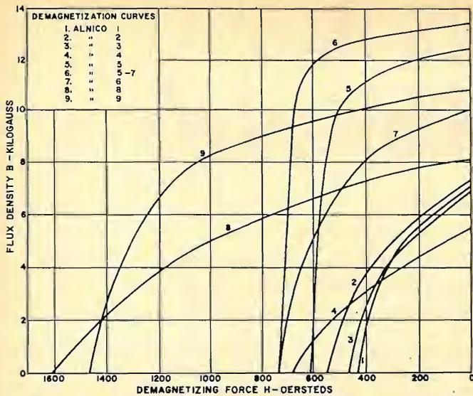
Fig. 3. Comparative demagnetization curves for various Alnicos.
