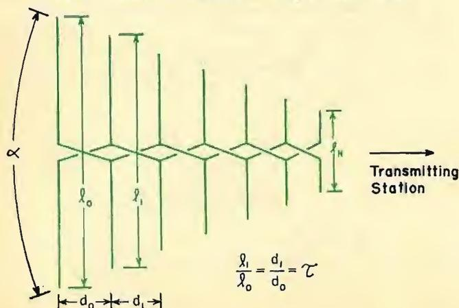
vertical space for installation and can be used in an attic with an inexpensive rotor to provide multi-direction reception. Finally, the solder connections to the center feeder line used in the original design have been eliminated, resulting not only in less work, but also in a better impedance match to standard 300-ohm line.
