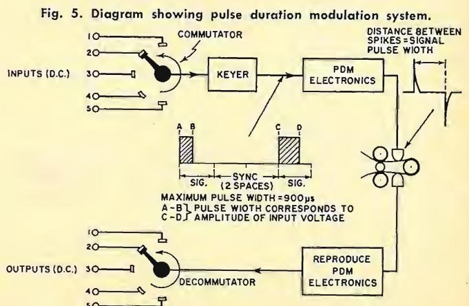
Fig. 5. Diagram showing pulse duration modulation system.
