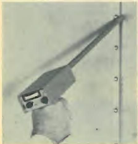
tions that can cause r.f. leakage at frequencies to 10 GHz and higher are readily detected.
