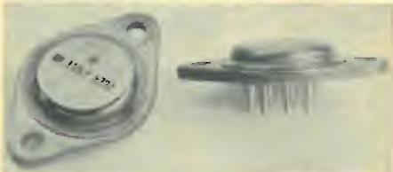
replace most present discrete power-supply regulators since these integrated circuits can deliver 0-2 ampere outputs at 8 to 48 volts. According to the company, they provide 2% or better regulation at 1 ampere.
