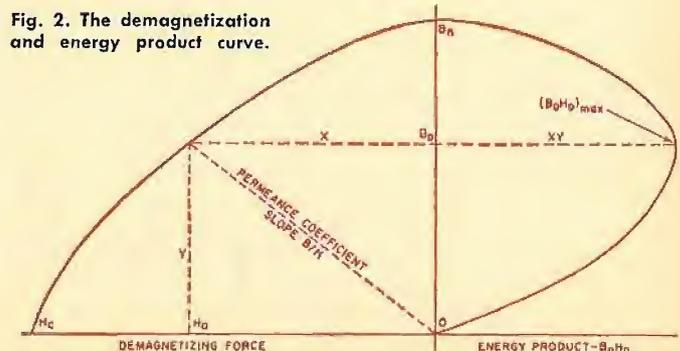
Fig. 2. The demagnetization and energy product curve.
