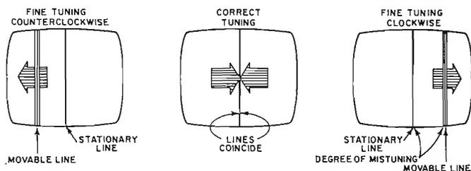
Fig. 1. Operating the fine-tuning control moves vertical line.
