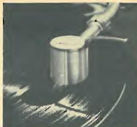
Operational theory of the cartridge is as follows: 1. the movement of the screen controls the amount of light ray passing through the screen on to the diode; 2. the movement of the stylus on the record causes the screen to vibrate; 3. the amount of light ray passing through the screen on to the diodes changes the current of the diodes to sound current. The cartridge, according to its maker, can transform the most minute vibration to electricity. Kenwood
