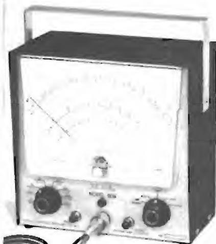
ALTHOUGH solid-state instruments are beginning to appear on dealers' shelves and on technicians' workbenches, many users still swear by the extremely simple, tried-and-true 6AL5-12AU7 circuitry of the conventional v.t.v.m.
